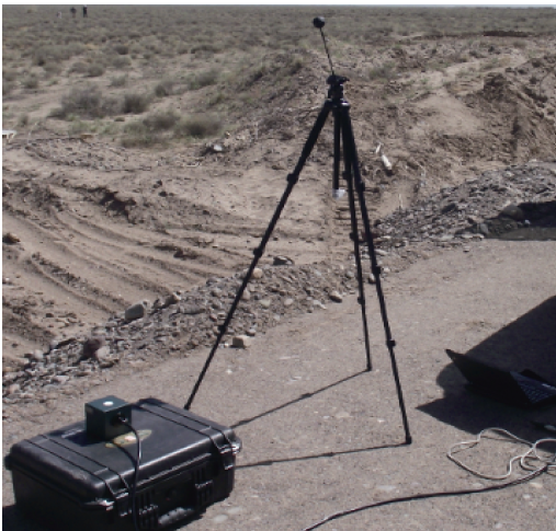
Figure 2 Measuring instrument of diffuse-to-global ratio
