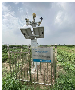
Figure 13 Ground monitoring system for burdock growth
