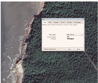
Figure 4 Difference between sea-land boundary of Google Earth image and the high-water line in rock shoreline of P. R. Korea (8 m)
