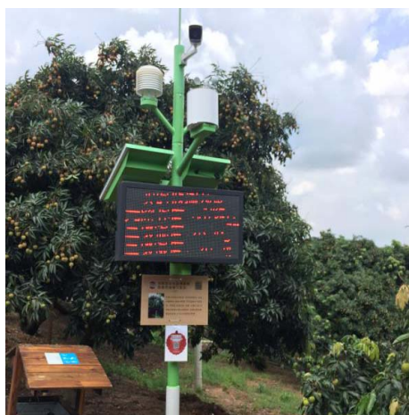
Figure 17 Monitoring station of Litchi Expo Park
