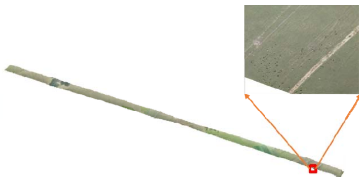
Figure 2 Example of a flight strip mosaicked with UAV image tiles
